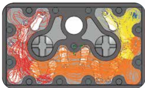
Previous cylinder cover – high pressure drops and turbulences
